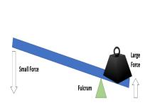
Can be used to make a small force lift a heavier load. A lever always rests on a pivot.
